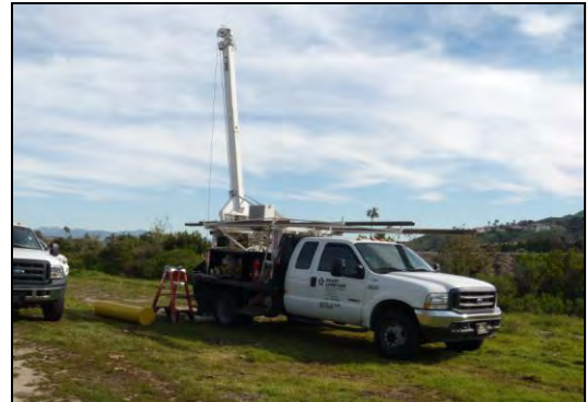
Pump Hoist Rig Used for Monitoring Well Development
