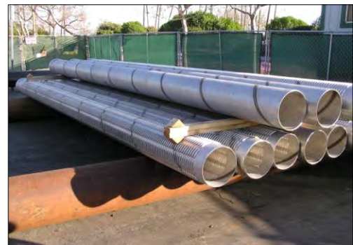
2507 Super Duplex Stainless Steel Casing and Screen
