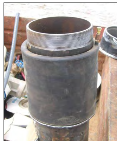
Inflatable Packer Used to Isolate Screen Intervals
