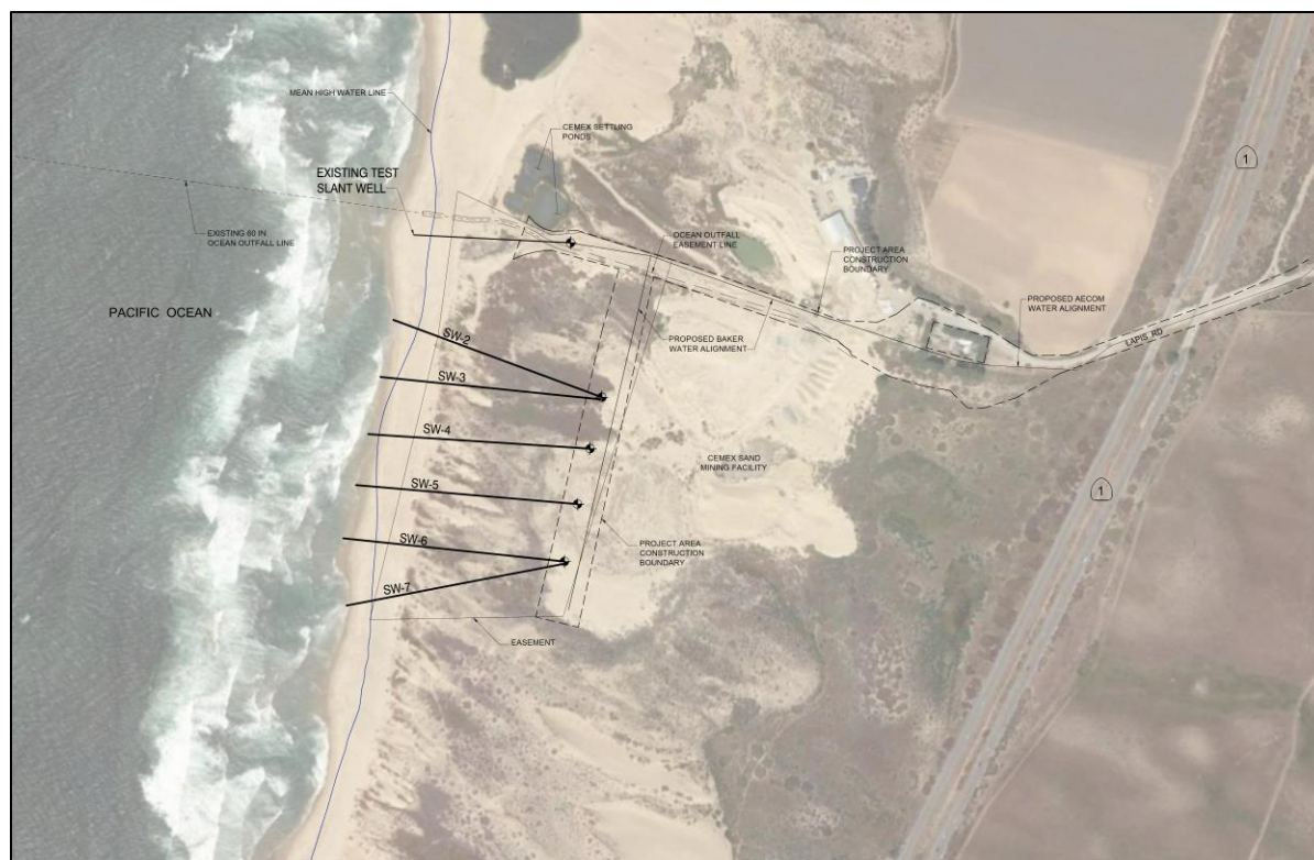
Figure 5-1. Proposed Full-Scale Slant Well Layout – 15.5 MGD Raw Water Supply
